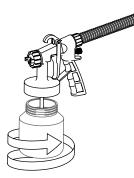
An airtight seal is essential for the correct operation of this spray gun. Before operating the unit please ensure that the paint container is securely fixed to the spray gun body and the gasket is in place.
